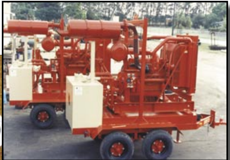
12" PUMP PORTABLE TRASH PUMP POWER UNIT
