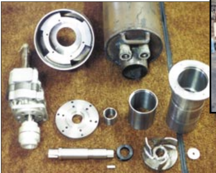
3" PUMP CUSTOM PUMP HEAD DESIGNED TO FIT IN 10" WELL CASING
