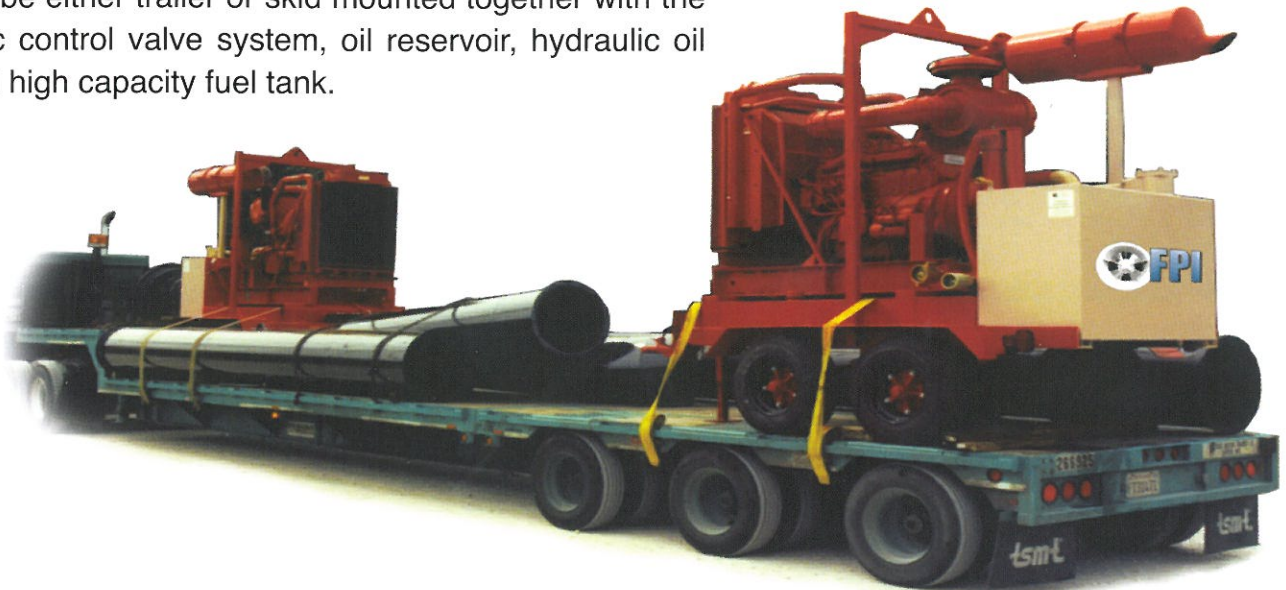
275 HP PORTABLE HYDRAULIC POWER UNITS WITH 30" DIA. HYDRAULIC PUMPS AND PIPING READY FOR SHIPMENT
